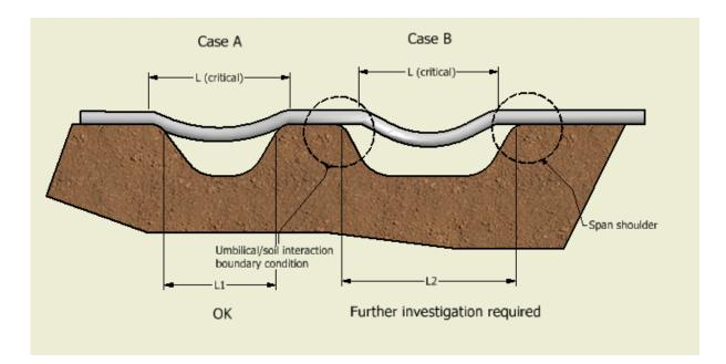
The reasons for the umbilical being unsupported can be various, e.g. local seabed topology, scouring of the soil from underneath the umbilical, the physical configuration of the subsea terminations, spans between I-tube and seabed, and at pipeline crossings.
